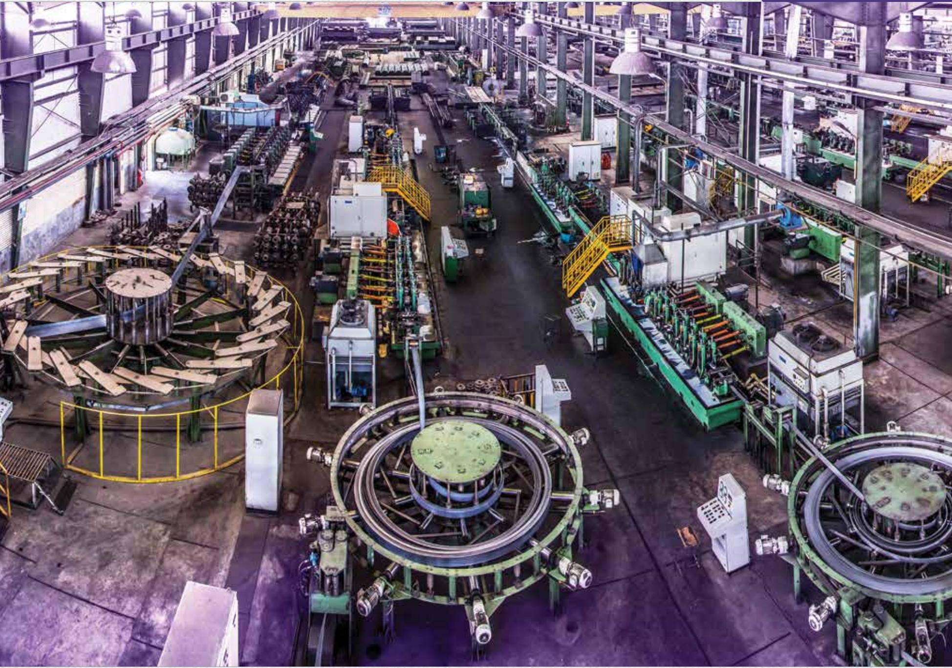
The production line of the ERW steel pipe from 3/8 to 6 inches
